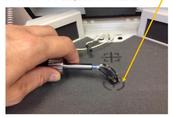
4. Set input to TL (Test-Loop) level at same value as before – in this case shown as 65dB. Run the TL test with the lid open - this will allow you to hold the instrument in the vertical or the "as worn on the ear" position.
