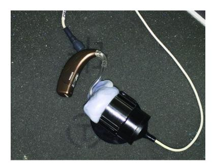
2. Make sure the instrument is set to Microphone – run the test using, in this case, 65dB speech input. Run the test with the lid closed.
